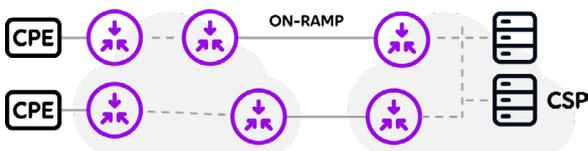
Option 3: Dual physical ports & cloud connections provide full redundancy from customer's network onward
