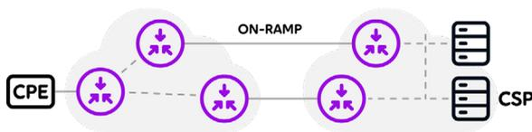
Option 2: A single physical port & dual cloud connections provide full redundancy from Telia Carrier's backbone onward.
