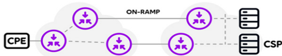
Option 2: A single physical port & dual cloud connections provide full redundancy from Telia Carrier's backbone onward
