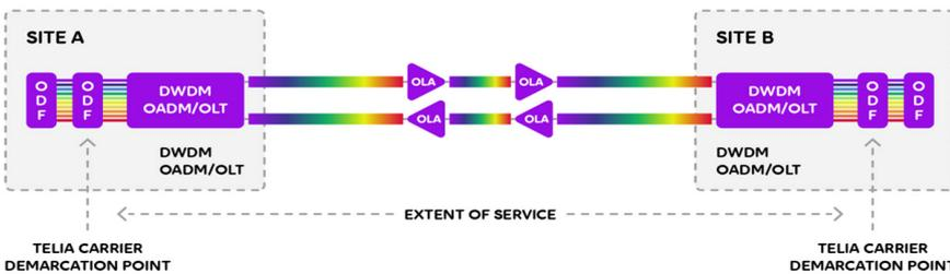
Figure 1: DWDM network components
